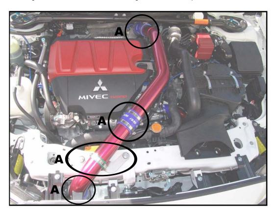
**Step 8: Removing the Stock Lower Intercooler Pipe (LICP)**
